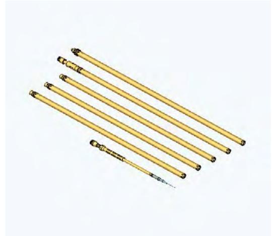
The small diameter Piezoprobe was designed to measure excess pore pressure and determine the dissipation characteristics of the sub-soils. In addition, results from the tests could be used to estimate the insitu permeability and consolidation characteristics of the soil, as well as provide insight into pile-soil set-up. The tool was made compatible with the Dolphin suite of in-situ tools to facilitate deployment.
