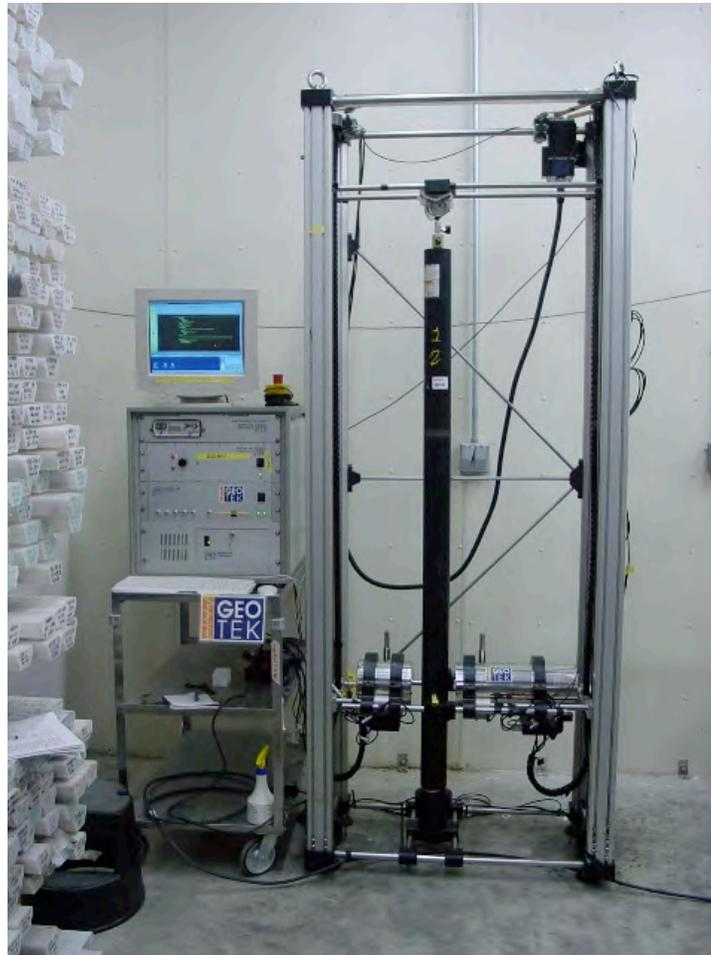
As a 'quick look' to determine the nature of the samples stored under pressure in the steel pressure vessels, the pressure vessels were subjected to gamma logging to determine the density structure. Logging took place at ODP using the GEOTEK vertical logging system during the period 7<sup>th</sup> to 14<sup>th</sup> October 2002. This was about 6 weeks after the samples had originally been recovered.
