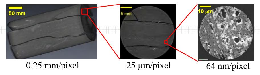
3D, multiscale X-ray CT scanning from core to nm scales.
