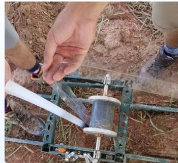
Field deployment. Fiber packaging for friction coupling to formation
