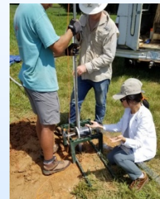
Field deployment. Fiber packaging for friction coupling to formation
