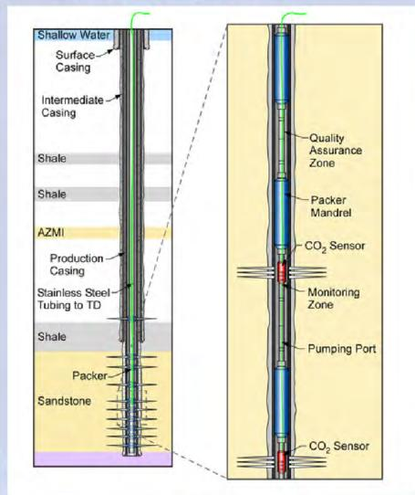
B) In porous "leak-monitoring" layer (above-zone monitoring interval (AZMI))
