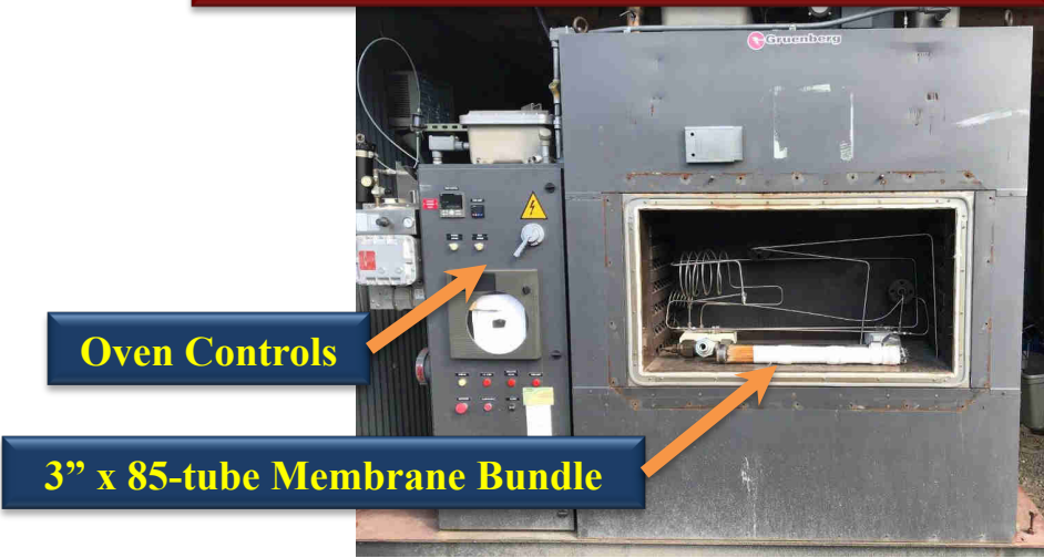
Front View: Oven Chamber with Membrane Test Module and a 3" x 85-tube Membrane Bundle for Perspective
