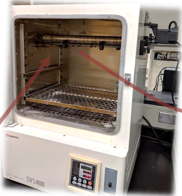
Rotated hydrothermal synthesis of long-tube MFI zeolite membranes
