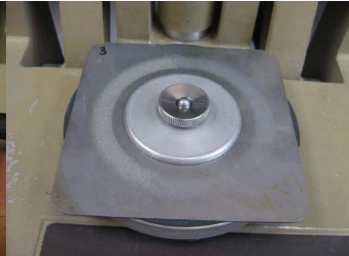
DragX™ Treatment (Mass Loss ~ 50mg/1000 cycles)
