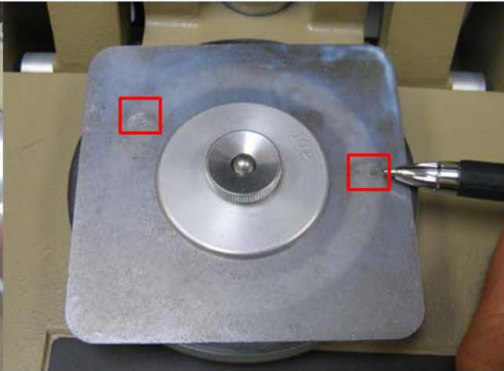
Poorly Adhered Coating (Mass Loss ~ 100mg/1000 cycles)
