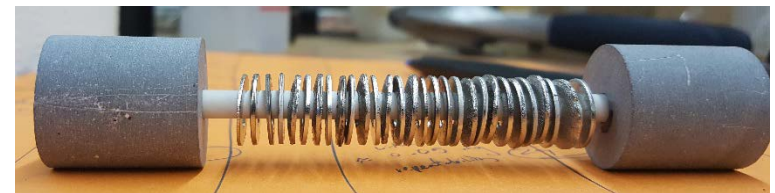
Washer Coupons on Support Rod
