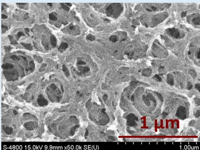
UKy-CAER developed Carbon Xerogel (CX) is a type of mesoporous electrode material
