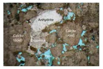
Williston basin reservoir rock thin section 40X magnification (Braunberger et al., 2012).
