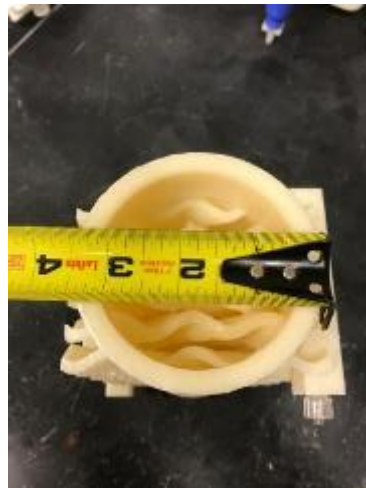
Design (left) and test print (right) for 3D printing ABS heat transfer packing material based on 250Y design from LLNL.
