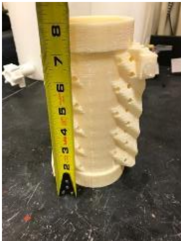
Design (left) and test print (right) for 3D printing ABS heat transfer packing material based on 250Y design from LLNL.
