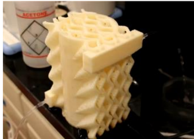
Design (left) and test print (right) for 3D printing ABS heat transfer packing material based on 250Y design from LLNL.
