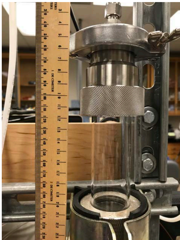
Small absorption column ~50 g material
