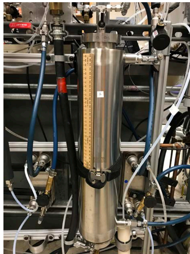
Larger, automated absorption column ~300 g material
