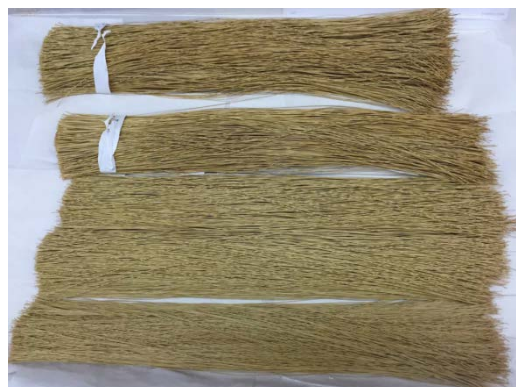
PBI hollow-fiber membranes Source: SRI
