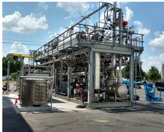
MTR small-pilot (1 MWe) membrane capture system Source: MTR
