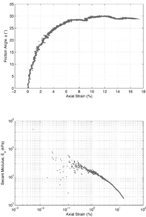
Figure 7. Effective friction angle and secant modulus vs. strain for NGHP-01 sample GH115.
