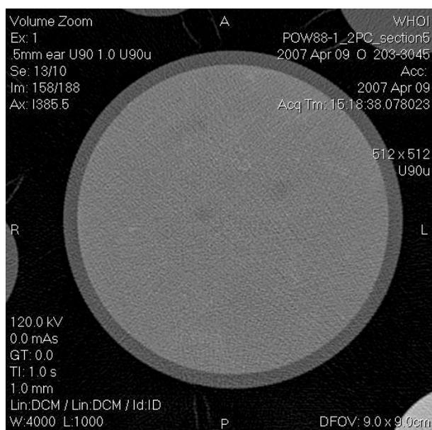
Figure 3. CAT-scan image of a refrigerated (+4°C) POW88-1 (Gulf of Maine) core section. Notice the uniform sediment structure prior to freezing.
