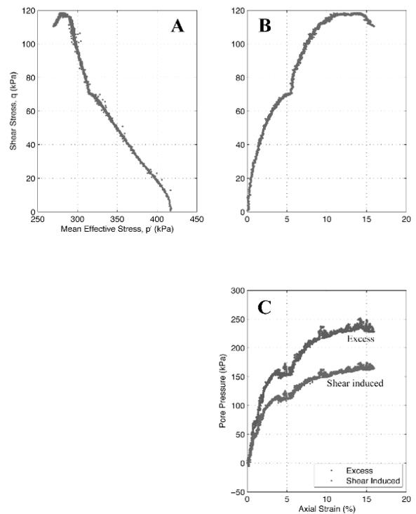
Figure 10. Shear strength results for NGHP-01 test sample GH117. Individual plots are (A) shear
