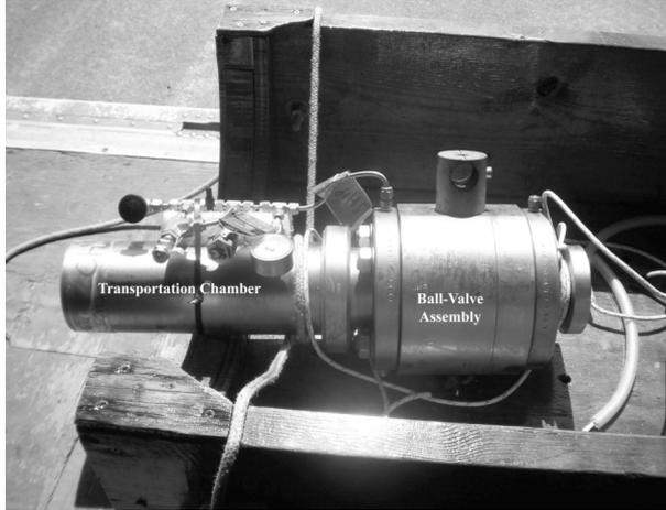
Figure 1. Pressure transportation vessel (smaller-diameter section at left) containing a NGHP-01 sample, sealed with a ball-valve assembly (larger-diameter section at right).
