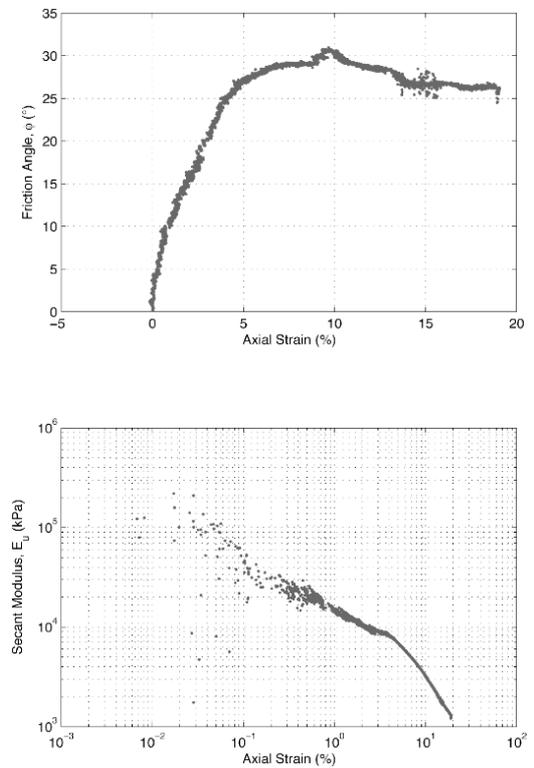
Figure 9. Effective friction angle and secant modulus vs. strain for NGHP-01 sample GH116.
