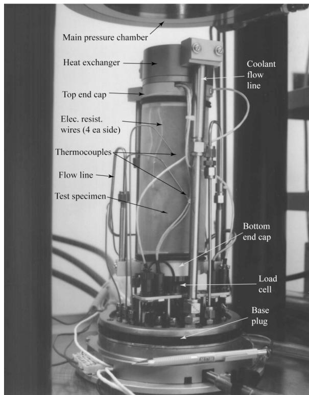
Figure 2. Close-up view of a test specimen about to be raised into the main pressure vessel (visible at the top of the photograph). The test specimen (gray cylinder) is located in the central part of the
