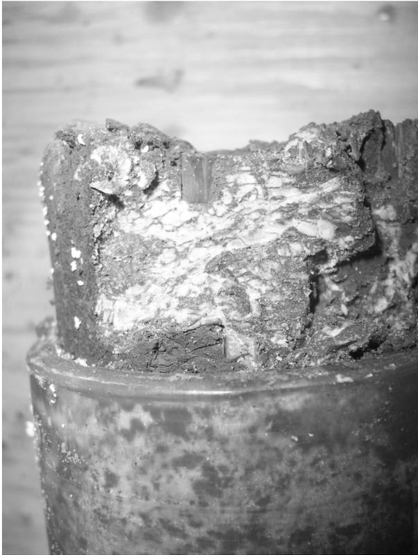
Figure 5. NGHP-01 sediment and gas-hydrate veins preserved within a refrigerated, methane-pressurized chamber.
