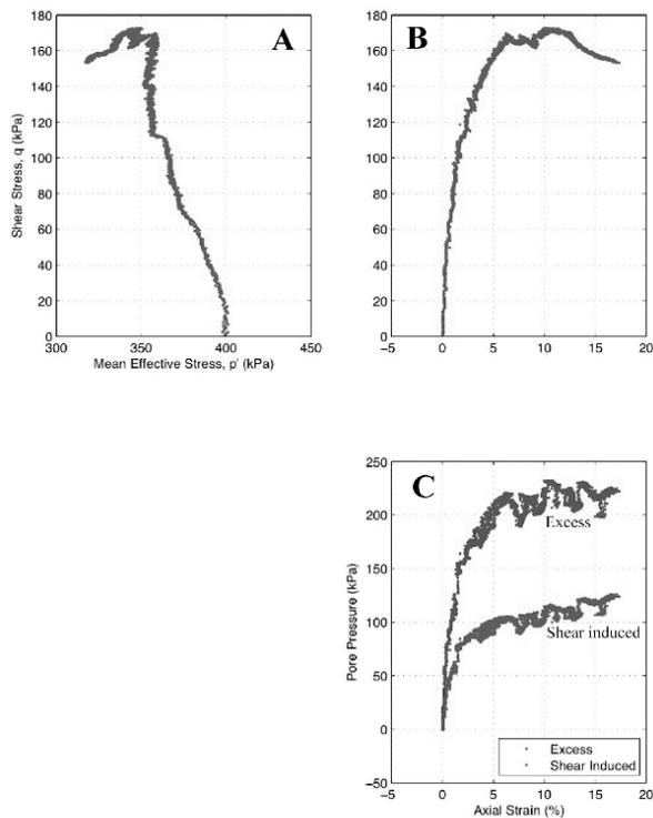
Figure 6. Shear strength results for NGHP-01 test sample GH115. Individual plots are (A) shear
