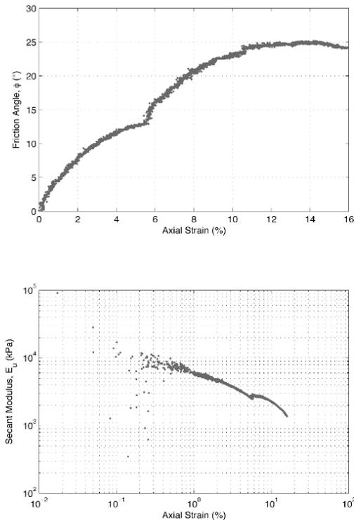
Figure 11. Effective friction angle and secant modulus vs. strain for NGHP-01 sample GH117.
