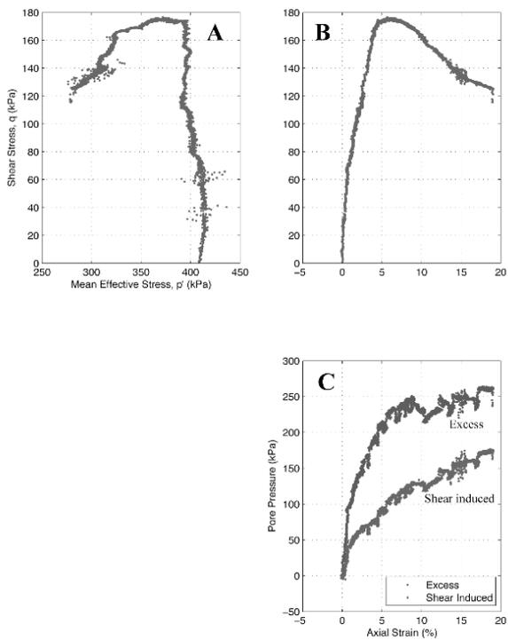
Figure 8. Shear strength results for NGHP-01 test sample GH116. Individual plots are (A) shear stress ( $q$ ) vs. effective normal stress ( $p'$ ) on a plane inclined at  $45^\circ$  from the horizontal. Each data point represents the top of a Mohr's circle and
