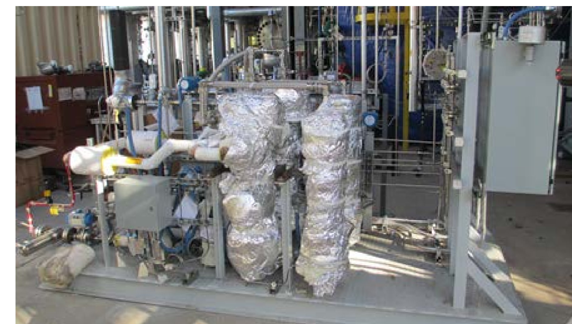
SRI's 50-kW th skid for 4-in module testing
