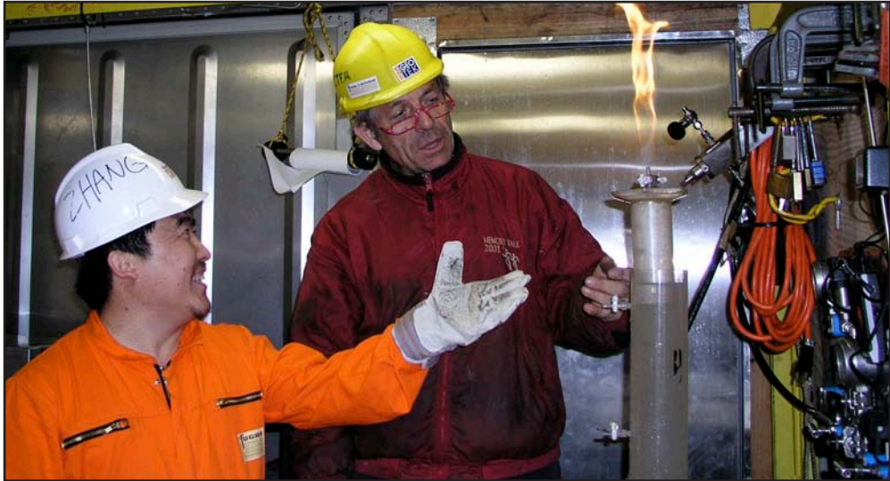
Drs. Haiqi Zhang and Peter Schultheiss show their excitement as a gas-hydrate-containing pressure core is slowly depressurized, releasing methane. The gas released is analyzed and quantified to obtain a mass balance for each pressure core, allowing the gas hydrate within the core to be accurately determined.
