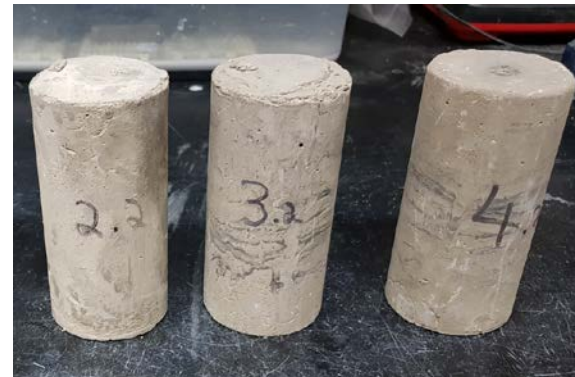
Cylindrical mortars having dimensions of 50 mm × 100 mm (d × h)
