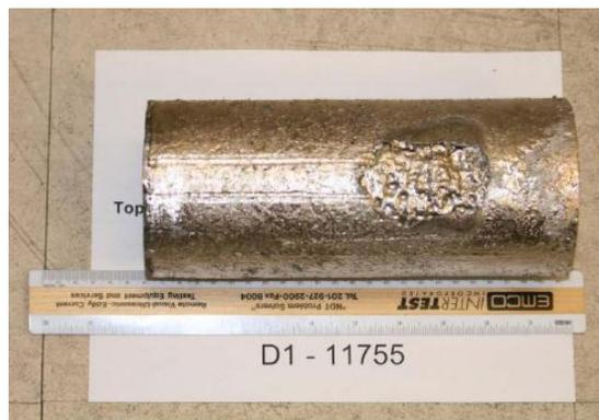
*Image of a 30 lb prototype steel ingot designed and produced by QuesTek*
