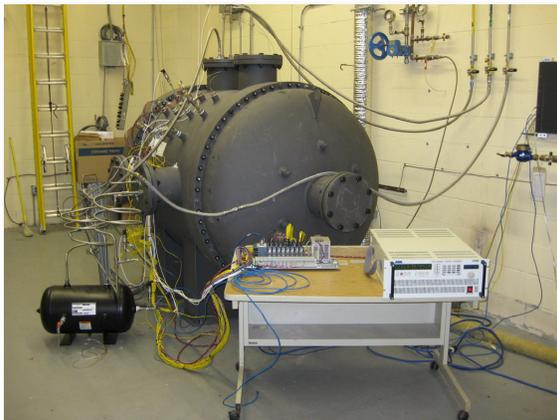
*Fifty-inch Inside Diameter Vessel for Pressurized SOFC Stack and System Demonstrations. Nitrogen/argon gas is supplied to the pressure vessel to balance the ambient stack pressure to the anode and cathode pressures. Algorithms will be used to simultaneously raise all zone pressures as well as continuously monitor and control all three pressures using a single set point.*
