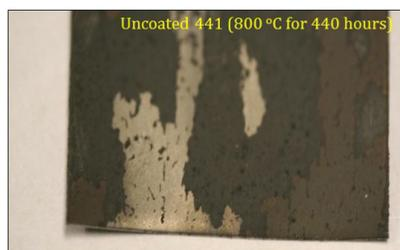
Images of ~1"x1" coupons of (Mn,Co)<sub>3</sub>O<sub>4</sub> coated and uncoated 441 SS following oxidation in ambient air at 800 °C. The coated scale remains adhered while large portions of the uncoated scale have spalled.
