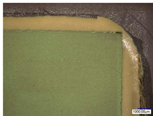
Post-test image of SCN-1 compliant glass sealed between aluminized AISI441 and an anode/electrolyte bilayer . No evidence of damage or leakage was observed after 12 thermal cycles between RT and 800 °C.
