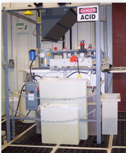
Photograph of pilot-scale electrodeposition cell for coating industrial scale SOFC interconnects.
