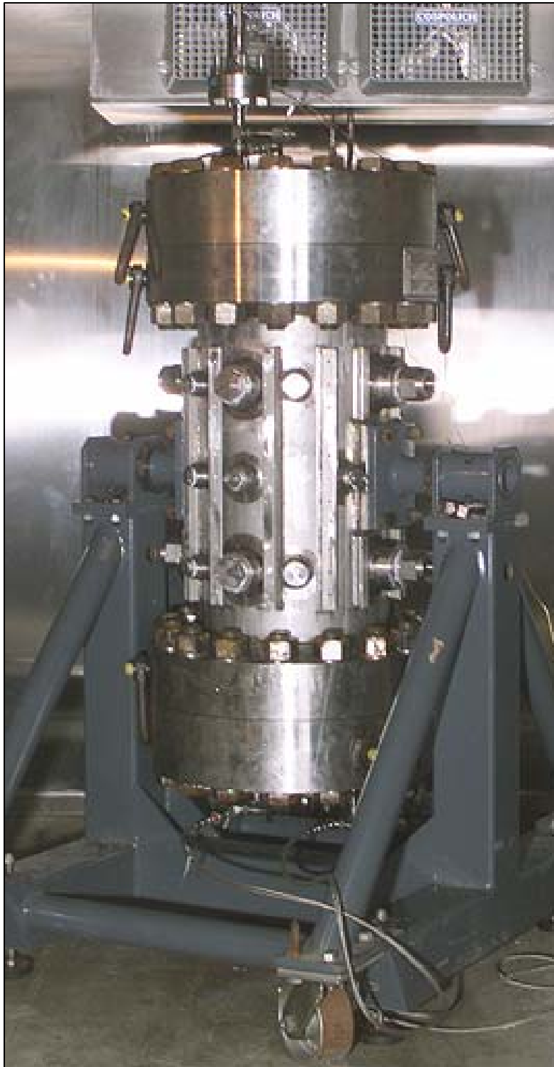
Figure 3. Oak Ridge National Laboratory's Seafloor Process Simulator is a cylindrical 72-L volume Hastelloy C- 22 vessel with 42 sampling ports, including 2 sapphire windows, that is capable of maintaining pressures up to 20 MPa.
