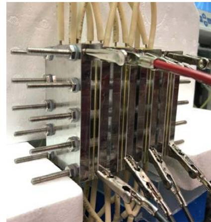
4 x 12.5 cm<sup>2</sup> (200 mA/cm<sup>2</sup>), 2M KOH electrolyte, Cu nanoparticles as cathode (loading at 1.2 mg/cm<sup>2</sup>), NiFe foam as anode
