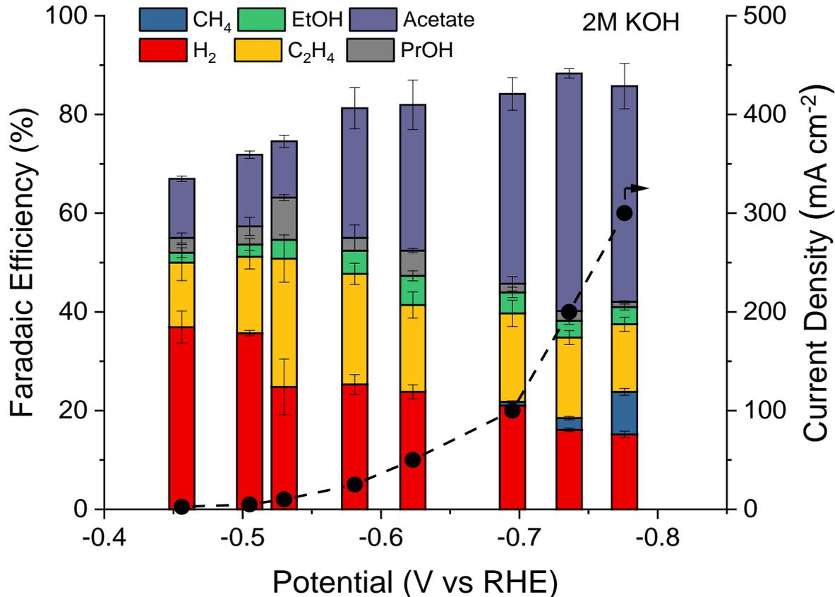
Cu(111) nanosheets exhibit a much higher acetate selectivity (up to 48%) than that of micron Cu and Cu nanoparticles (less than 25%).
