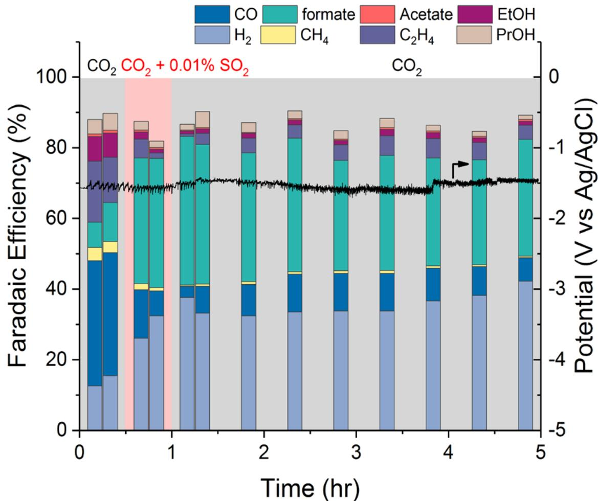
C<sub>2</sub>+ selectivity cannot be fully restored after 0.01% SO<sub>2</sub> exposure.
