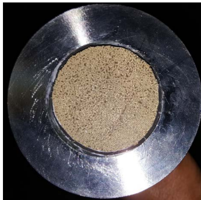
Potted 4-in fiber module cross-section (early design)
