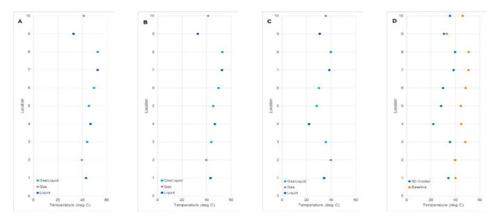
Plots of absorber temperature profiles for (A) baseline packing, (B) printed packing uncooled, (C) printed packing cooled, (D) comparison of baseline and cooled packing. The lean solvent feed is at location 9 and the flue gas inlet is at location 2; these are controlled temperatures.
