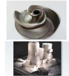
*As metallic additive manufacturing technologies matured, it became possible for complex metal product to be manufactured by this innovative technology, which also provides great capabilities to make complex geometries for turbine airfoil cooling channels.*
