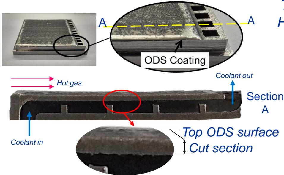
Coating layer intact after exposure to 1100°C to 1200°C main gas flow for ~24 hours.
