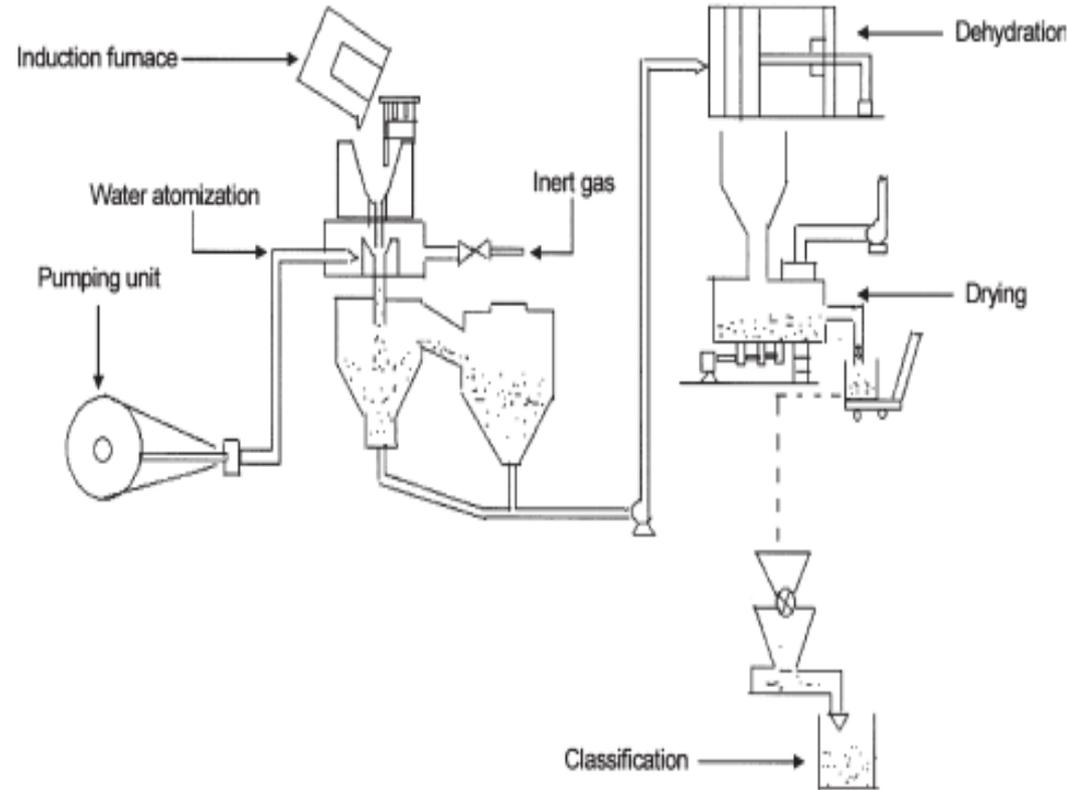
A schematic of Water Atomization
