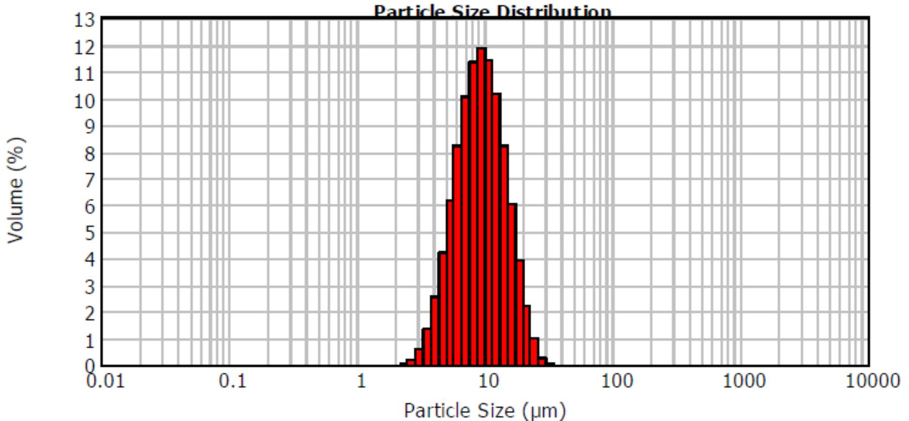
$D(0.1)=5.153\mu\text{m}$ ,  $D(0.5)=9.261\mu\text{m}$ ,  $D(0.9)=16.296\mu\text{m}$
