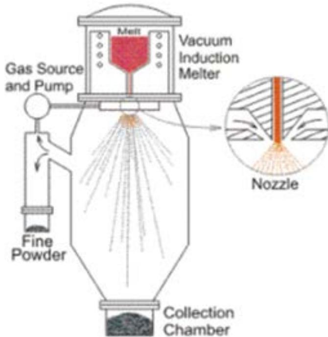
A schematic of Gas Atomization
