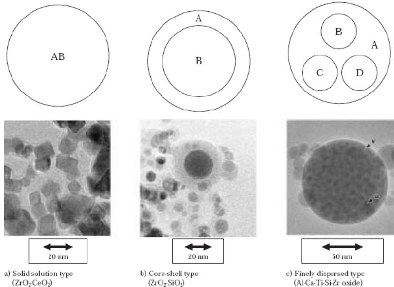
Structural patterns of nanocomposite particles
