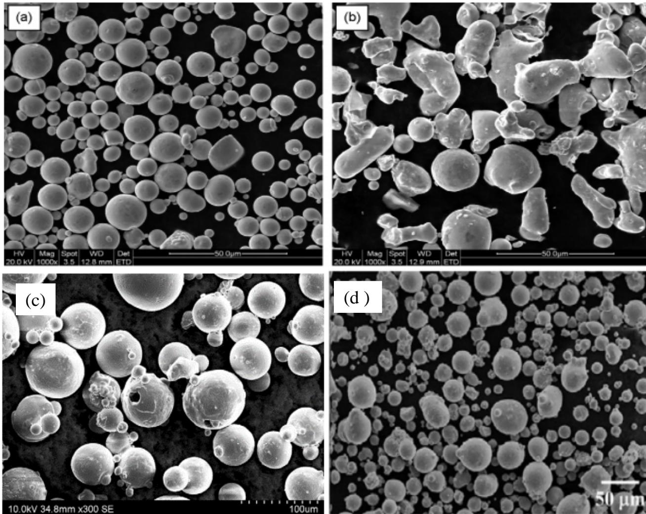
SEM images showing characteristic morphologies of Atomized powder: (a) gas atomized 316 stainless steel; (b) water atomized 316 stainless steel; (c) gas atomized Ti-6Al-4V; (d) gas atomized IN718
