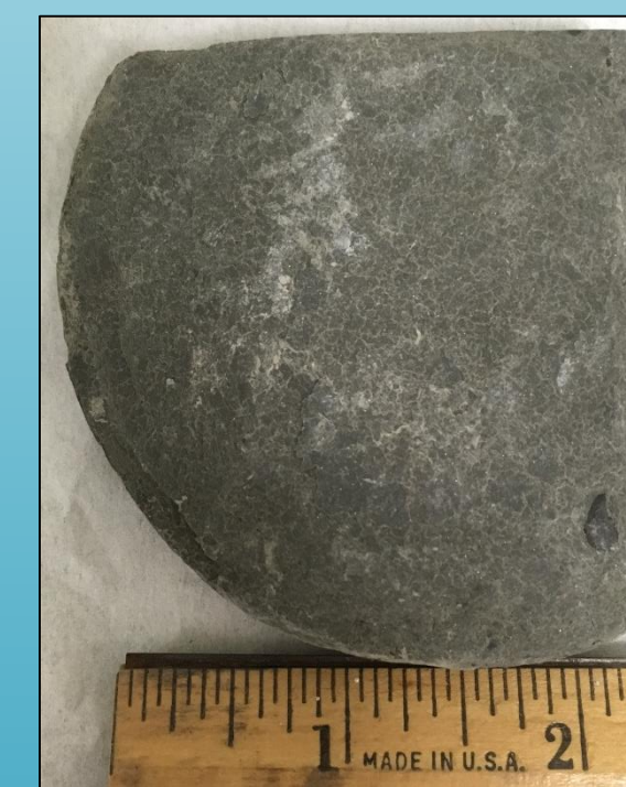
Top: Stratigraphic column of the FutureGen site showing the Mt. Simon Sandstone (CO 2 storage reservoir) and Eau Claire Formation (CO 2 sealing formation). Right: Eau Claire core.
