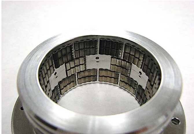
Installed Radial Bump Foils
