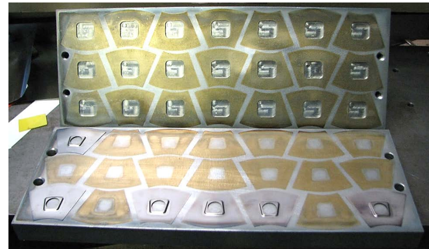
Heat Treat Plates with Processed Thrust Top Foils
