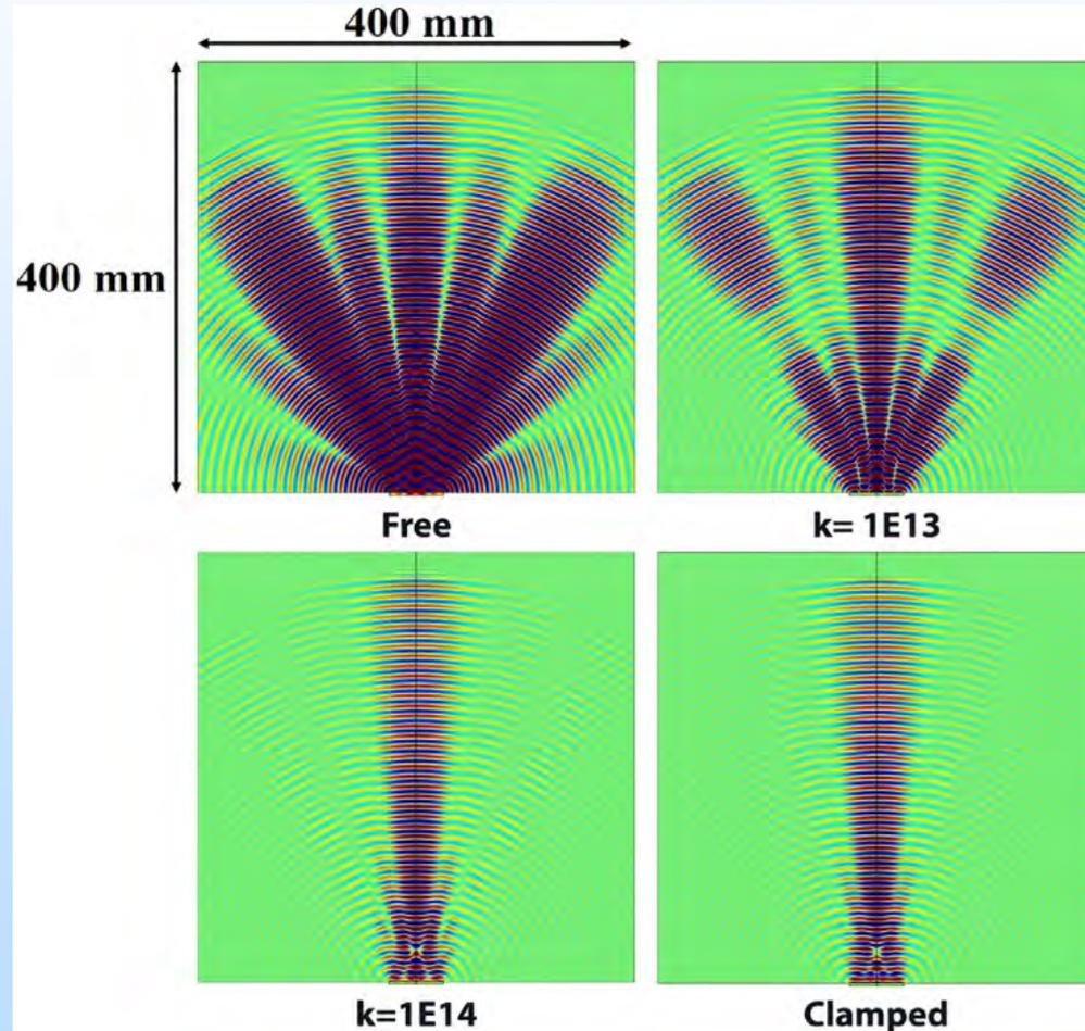
Normalized out-of-plane displacement on the surface of the disc for RM-3 for different lateral stiffness  $k$  (N/m<sup>3</sup>)
