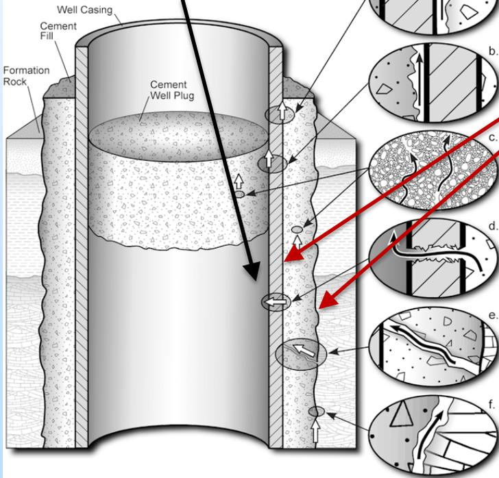
Extend applicability to: (1) casing-cement interface, (2) cement-formation interface, and (3) out in the formation (up to ~ 3 meters).
