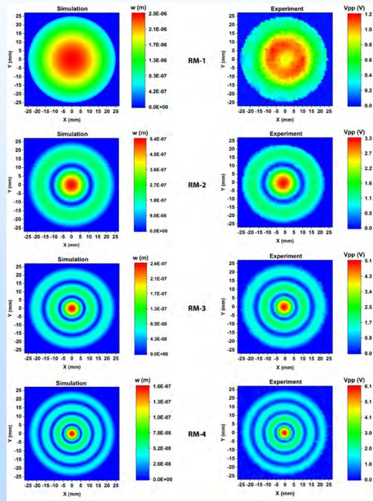
Comparison of analytical and experimentally obtained beam profiles from the radial modes
