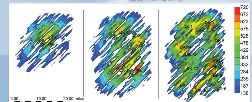
Figure 5. Simulated pressure plumes (in plan view) for the P90, P50, and P10 models (from left to right) at the end of a simulated 25-year CO<sub>2</sub> injection operation. The lower limit in pressure scale is bounded by the pressure threshold value of 138 psi. The pressure plume dimensions measure approximately 20x20, 21x30, and 22x32 miles, respectively.
