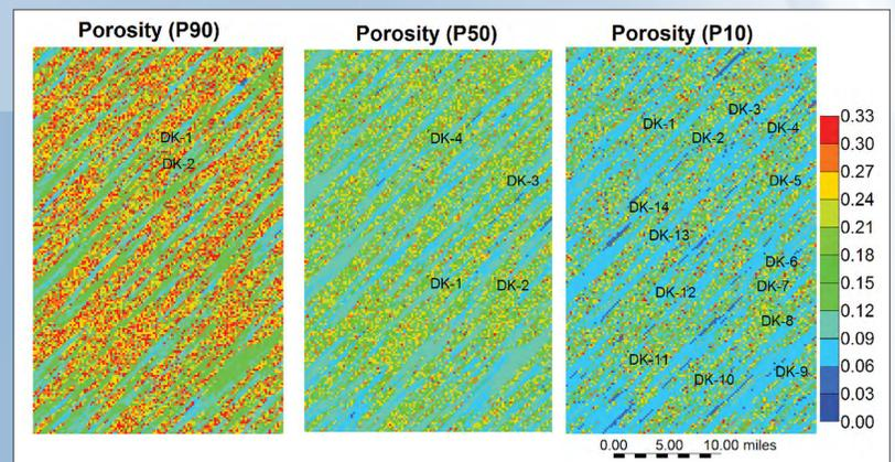
Figure 1. Porosity distributions (in plan view) with the potential well locations for CO<sub>2</sub> injection for P90, P50, and P10 models (from left to right). The injection wells are labeled "DK" (Dakota).
