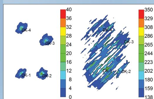
Figure 7. The postinjection CO<sub>2</sub> plume (in plan view) after 100 years of postinjection (left) and pressure plume extent after 40 years of postinjection (right).
