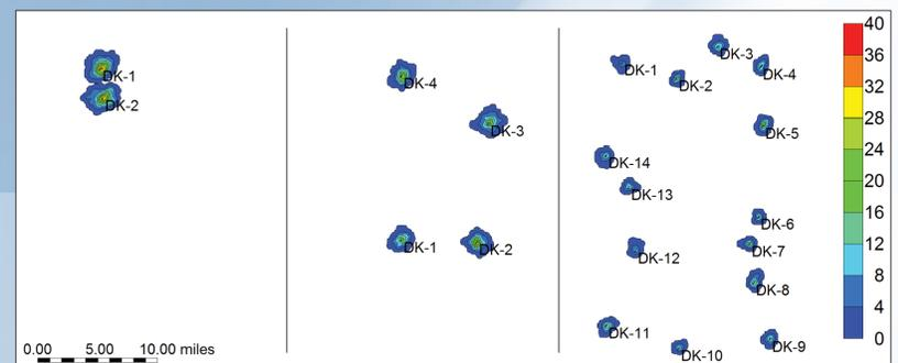
Figure 4. Simulated CO<sub>2</sub> plumes (in plan view) for the P90, P50, and P10 models (from left to right) at the end of a 25-year CO<sub>2</sub> injection operation. CO<sub>2</sub> per Unit Area = CO<sub>2</sub> Saturation × Porosity × Thickness. The CO<sub>2</sub> plume diameters measure approximately 3.5, 3, and 2 miles around each injection well, respectively.
