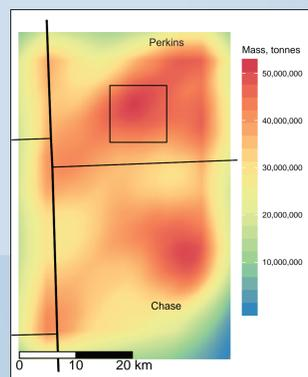
Figure 3. Simulation model volumetric CO<sub>2</sub> storage potential estimate in the Cloverly Fm within a 6.2-mile (10-km)-square moving window (size denoted by square in Perkins County). The color of each grid cell represents the amount of storage potential within a square window centered on that cell.
