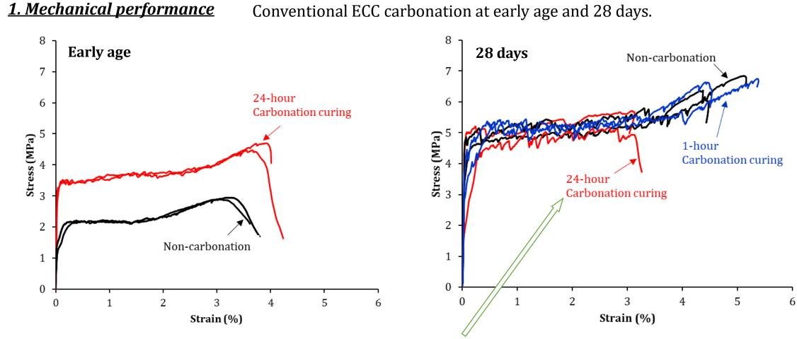
Carbonation curing accelerates early-age development of tensile strength and strain capacity. • At 28 days, carbonation-cured ECC achieves comparable tensile strength but slightly lower tensile strain capacity.
