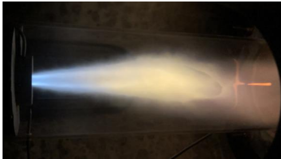
Photographs. 50kW,1.1bara, 538K. Heavily cracked conditions.
