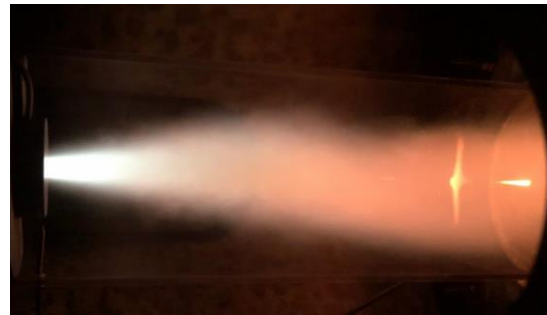
Photographs. 50kW,1.1bara, 538K. Heavily cracked conditions.
