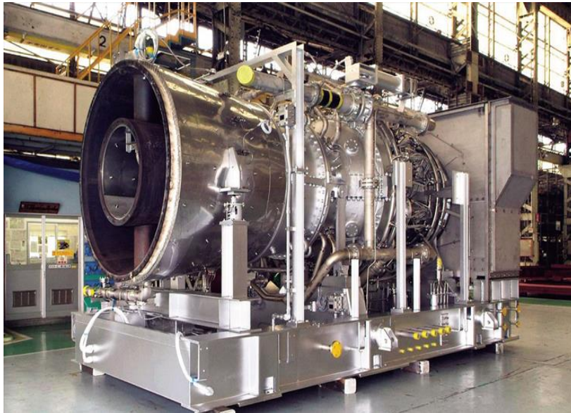
First Ammonia Gas Turbine Engine, MHI (H25), 40 MW Power [ https://power.mhi.com/news/20210301.html ]
