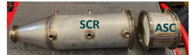
Experimental aftertreatment system
