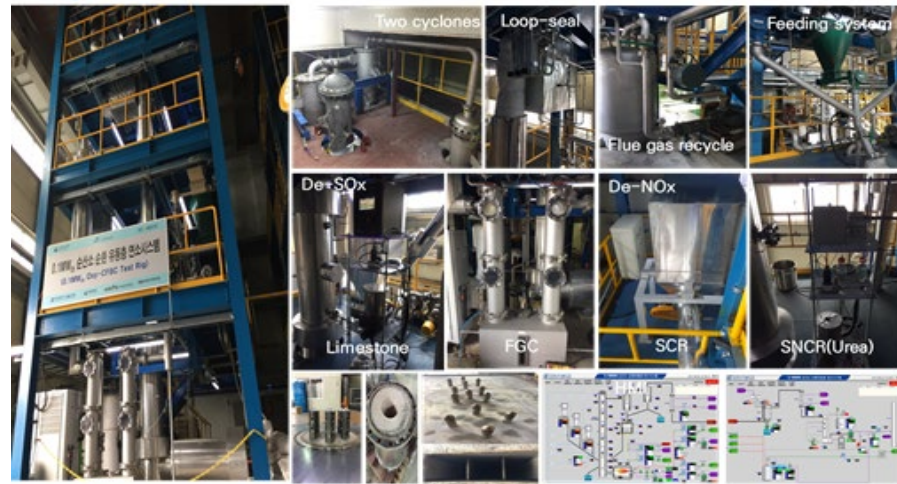
「 100 kW NH 3 co-firing CFB system 」
