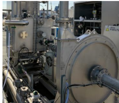
Double wall ventilation and absorber
