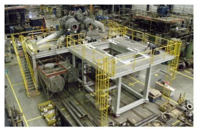
Siemens has built and tested LP and HP CO<sub>2</sub> supersonic compressor units at a size necessary for 90% capture at 182MWe (Award FE0026727)
