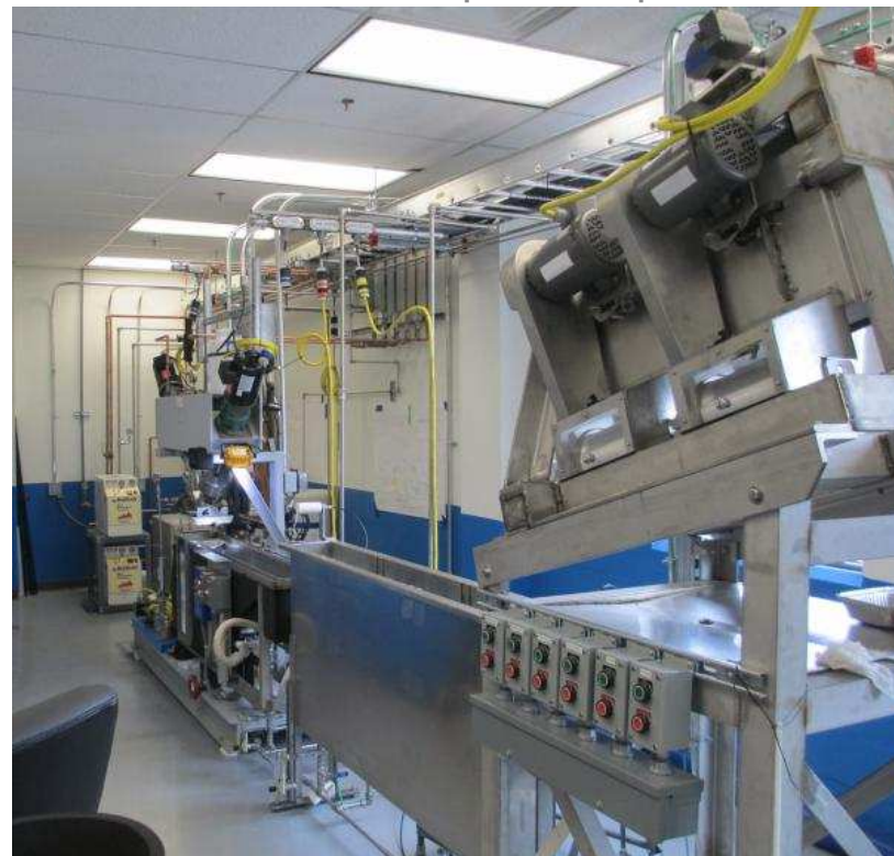
12-filament Development Spin Unit
