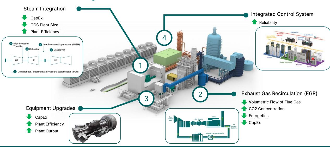
Integrated NGCC+CCS solutions can improve NGCC efficiency & reduce CCS cost (CapEx & OpEx)
