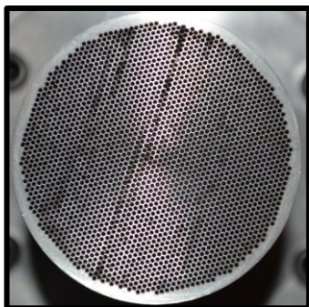
Burner Surface ~2400 holes, D=0.020 "
