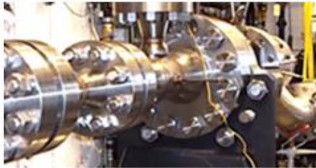
– Single-nozzle high-pressure combustor, fired w/ \text{NH}_3 fuel
