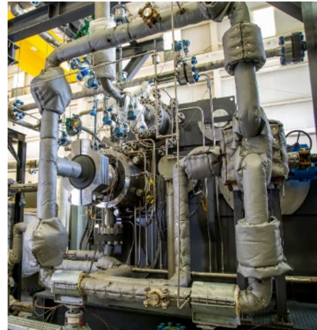
5.6 MW sCO 2 system and turbomachinery prototype (DOE, Hanwha)
