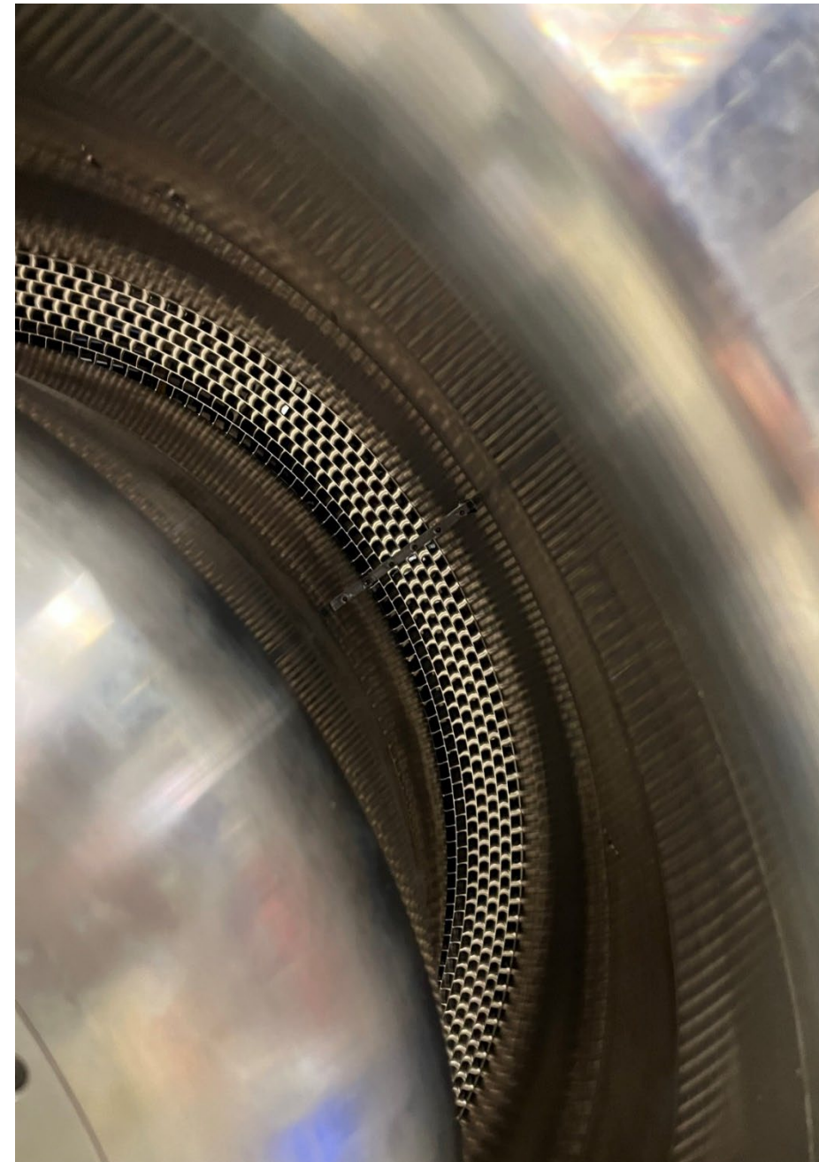
Inlet pressure rake upstream of flow-conditioning gauze.
