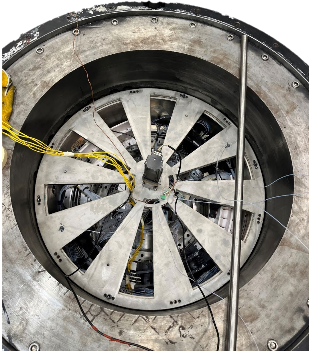
Sonic plate actuation downstream of the test section allows for modulation of flow rate/Reynolds number.
