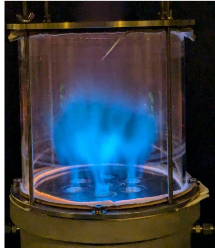
All Injectors 400 F preheat \phi = 0.81 \Delta P/P = 3\%
