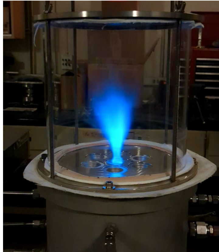
Center Injector 400 F preheat \phi = 0.98 \Delta P/P = 3\%
