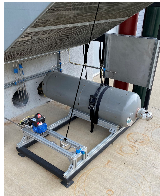
Relief valve calibrated to 225 psia
