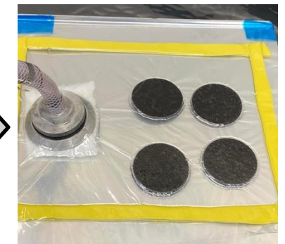
This 'densifies' the composite and reduces porosity
