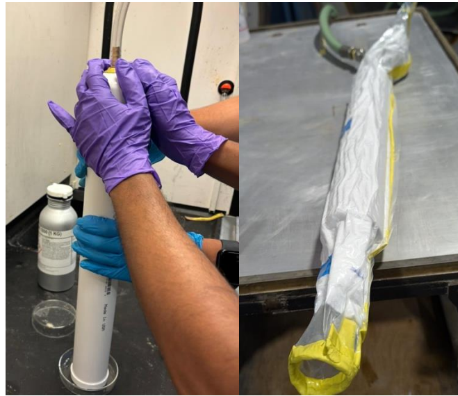
Resin infiltration and curing of the green body
