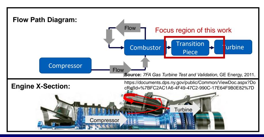
RDC combustor adds significant unsteadiness to flowfield that is not accounted for in current turbomachinery designs.
