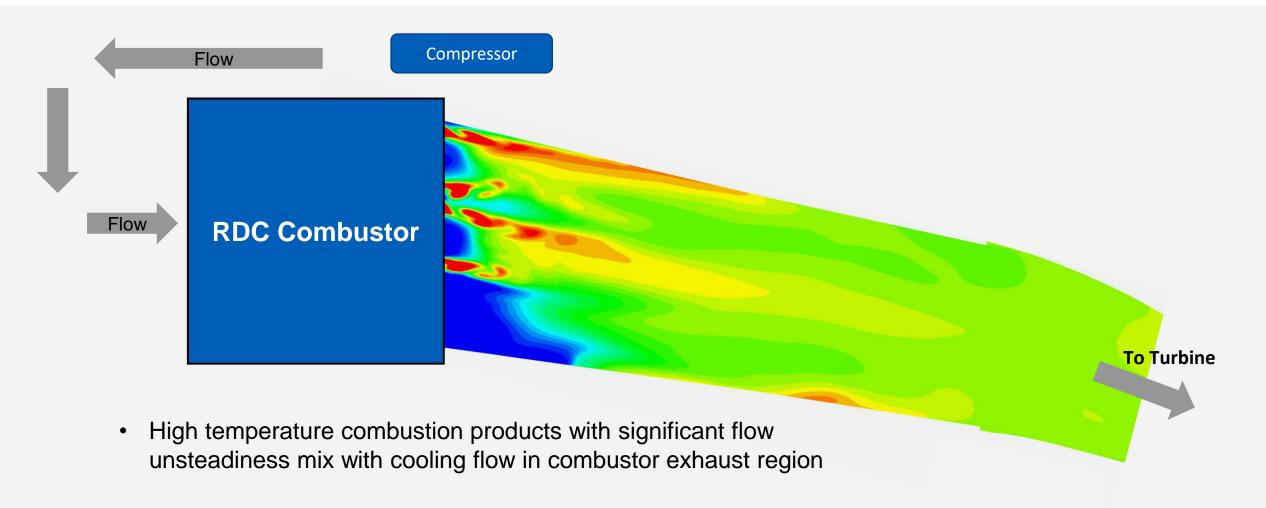
Hot gases mix effectively with cooling flow prior to reaching turbine section.
