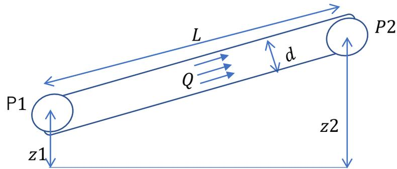
$Q$  = volumetric flow ( $m^3/s$ ),  $P$  = pressure (Pa),  $z$  = elevation (m),
