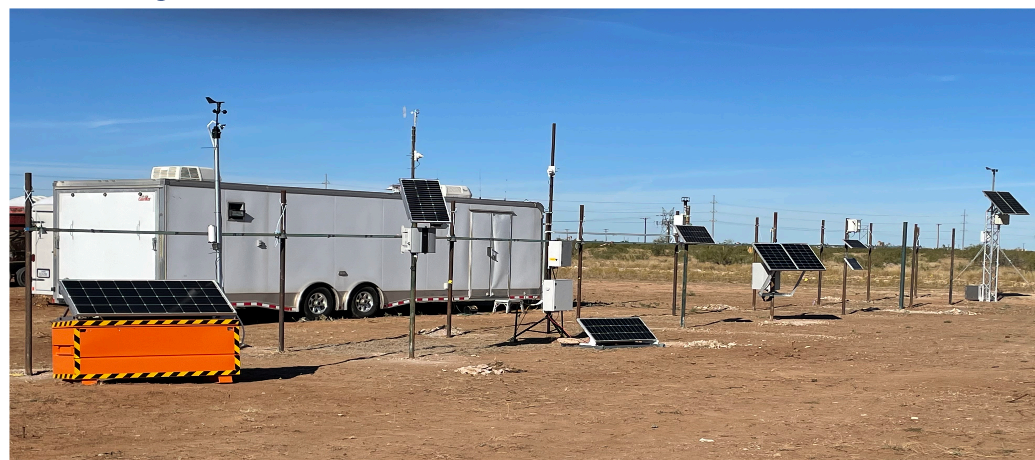
Figure: Project Astra methane sensor inter-comparison site in the Permian Basin
