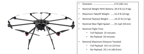
Figure 12. Aurelia X8 photograph and specifications.
