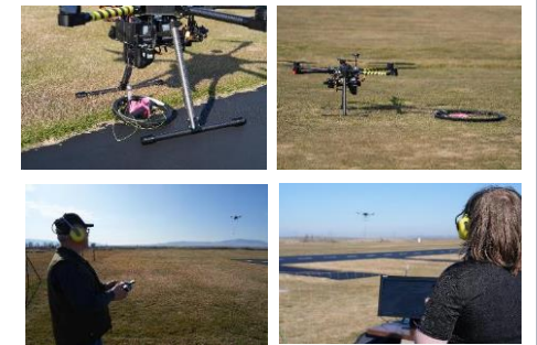
Figure 11. Photographs of UAS field tests using 'dummy' geophysical payloads consisting of transmitter and receiver coils without electronics. A winch is used to control the drone-antenna offset.
