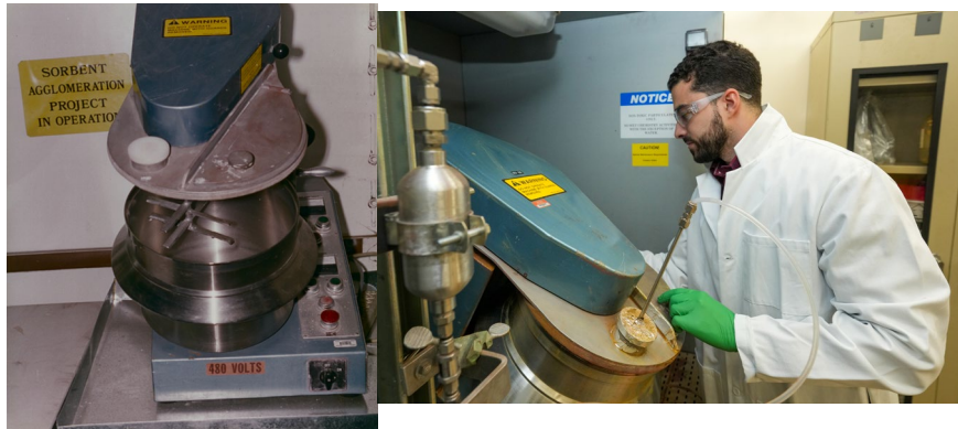
Catalyst preparation facility - Prepares <10 Kg quantities
