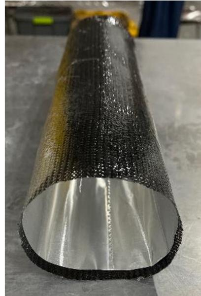
Resin-infused biaxial carbon fiber composite layer
