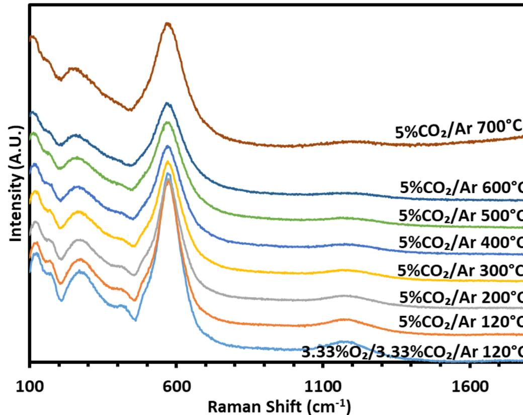
Oxidation with 3.3% O<sub>2</sub> re-created 4+ defects and exposure with CO<sub>2</sub> and Ar didn't show significant changes
