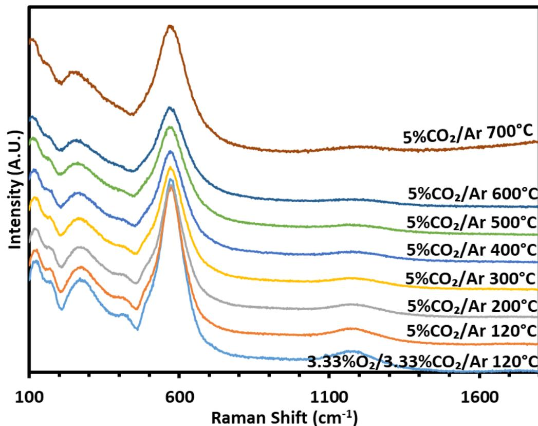
$5\%\text{CO}_2/\text{Ar}$  treated  $\text{Li}_2\text{CO}_3/\text{LaPrO}_3$  at  $120^\circ\text{C}$
