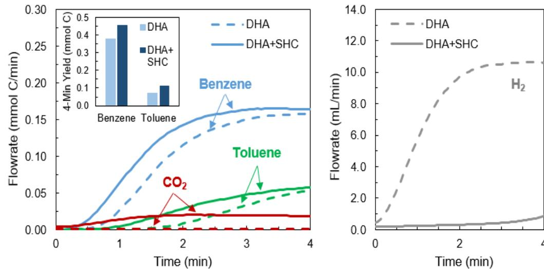
Effect of SHC redox catalyst on DHA in a sequential bed configuration
