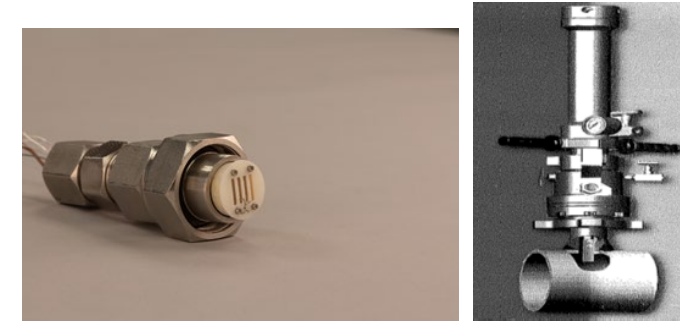
An AES prototype for simultaneous monitoring of corrosion rate, environment humidity, and temperature. (right) Example of an AES installation in a natural gas transmission pipeline.
