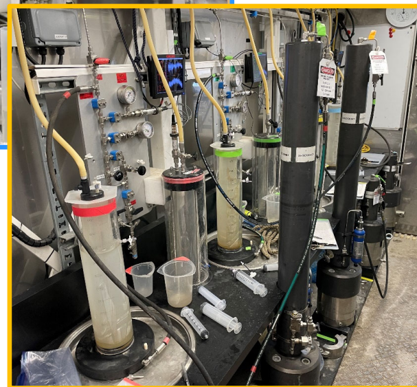
Geotek degassing container with 4 degassing stations
