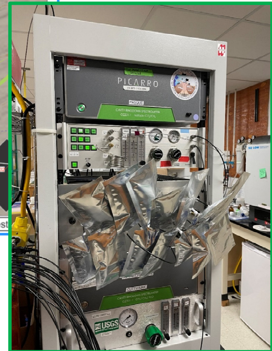
USGS Auto-SIM with in-line gas chromatograph analyzing GOM2-2 gas samples
