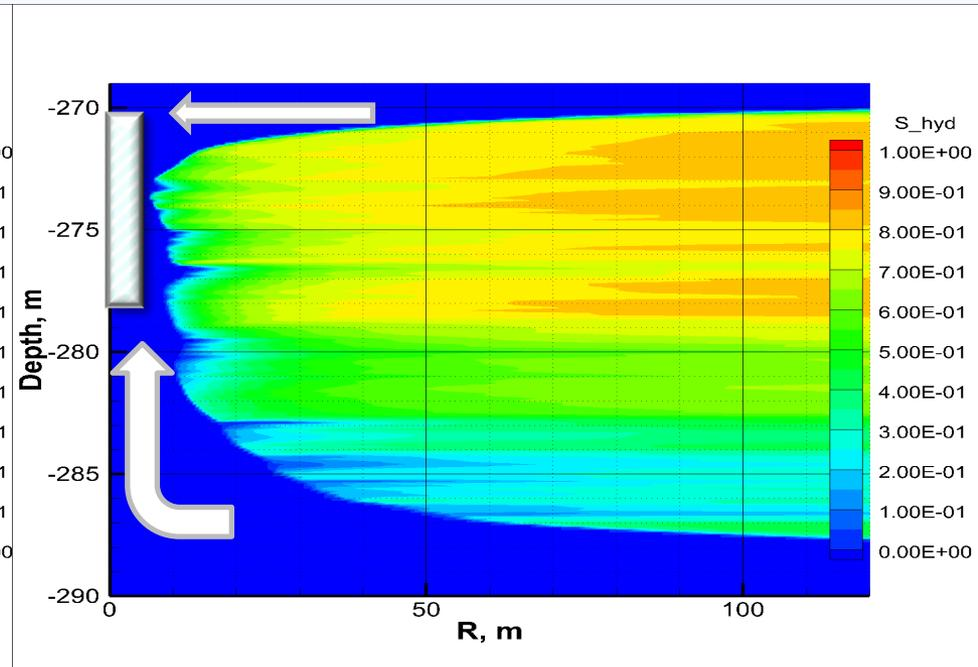
The balance between influxes from over- and underburden determines overall water production at the wellbore
